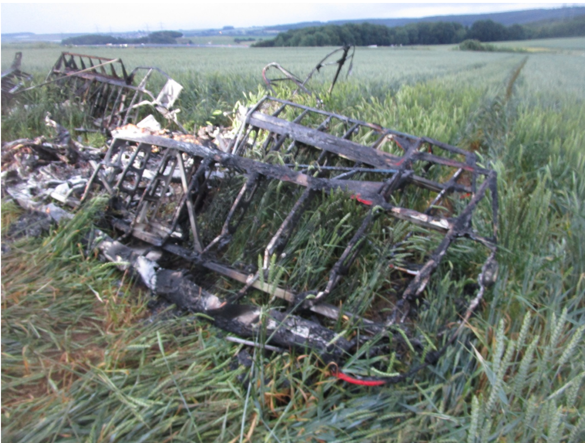
Fig. 16: Accident site after uncontrolled flight attitude Murphy Aircraft / Renegade 472 912 ULS Source: BFU
