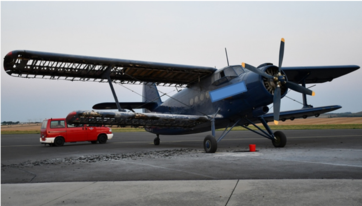
Fig. 6: Fire damage on the Antonov An-2
