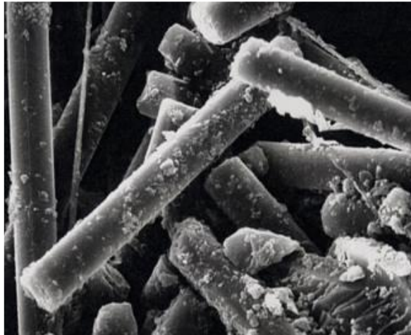
Fig. 45: Burnt carbon fibre debris (microscopic picture)
