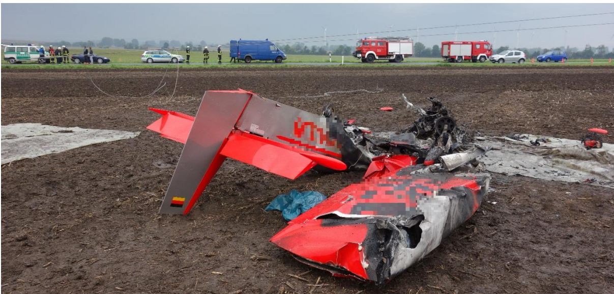
Fig. 26: An ultralight collided with a 20 kV power line in about 9 m high, one pylon was broken off and another damaged (hanging cables in the background)
