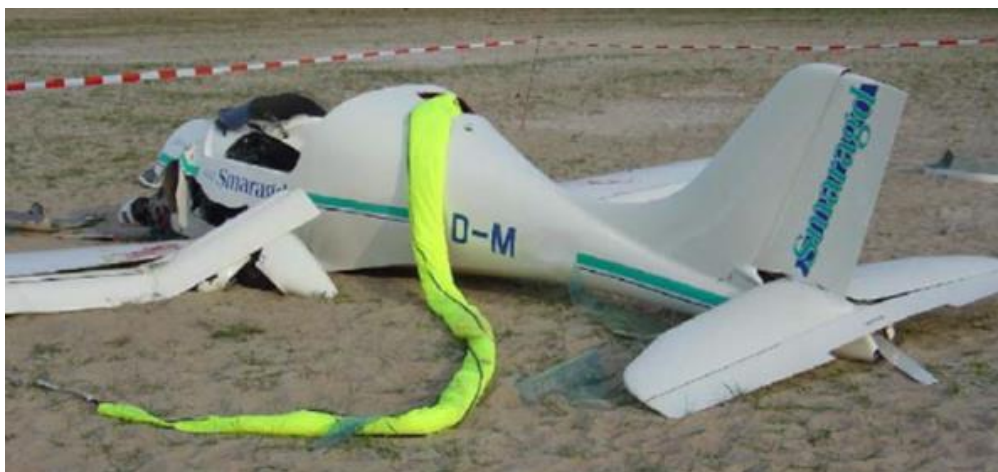
Fig. 44: Incomplete opening of a BPRS
