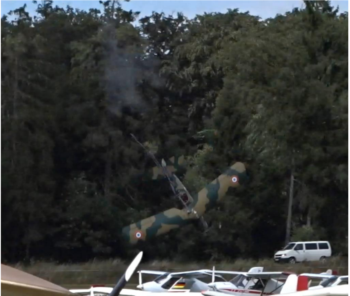
Fig. 43: Activation of the BPRS in low altitude
