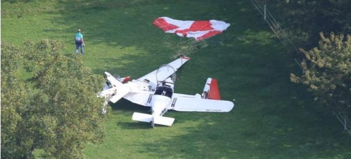
Fig. 42: BPRS activation after collision of an ultralight and a glider on final approach
