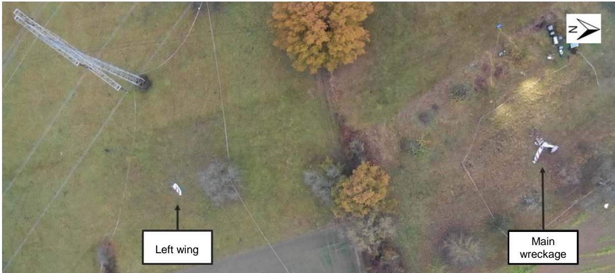
Fig. 27: Wing structure failure of an ultralight in-flight
