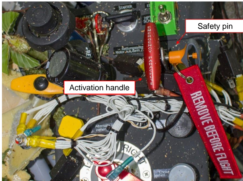
Fig. 41: Safety pin still securing the activation handle of the BPRS in an accident ultralight
